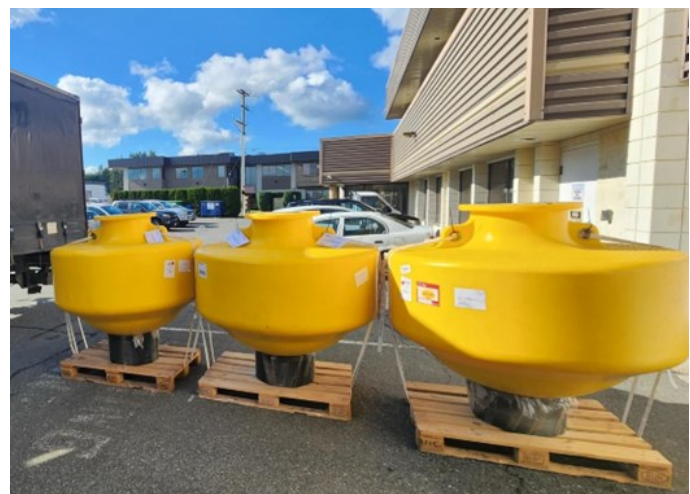
Figure 2. ASL has received three yellow buoys (the standard cautionary buoy colour) and are instrumented with a yellow flashing light to conform to the standards and guidelines in the Canadian Aids to Navigation System (TP 968).
