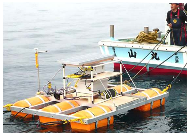
Test mooring of raft-mounted AZFP equipped with cellular modem used to study zooplankton in the water column, Yamada Bay, Japan, June 2016.
