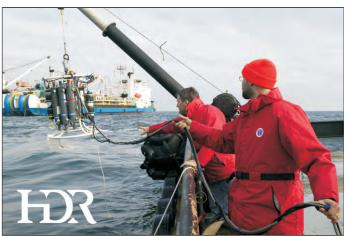
profiles and trigger the collection of water samples for suspended sediment plume monitoring. In addition, multiple OBS units were also used with fixed buoy arrays to continuously record turbidity at various water depths to monitor the spatial extent of suspended sediment plumes.
