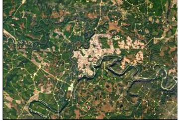
The image was acquired by the LANDSAT 8 satellite in 2013 and shows various types of disturbed areas, including clearcuts, oil and gas drill pads, pipeline corridors, and mines (Central Alberta, Canada).
