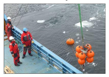
ASL is concluding an ice and metocean measurements and analysis program off NE Greenland for the Norwegian University of Science and Technology (NTNU) and Statoil. ASL personnel aboard the Norwegian Polar Institute's ship, the *RV Lance*, recently recovered the 4 Ice Profiler/ADCP moorings from Fram Strait. ASL is now processing the data from this second and final year of a very successful program.
