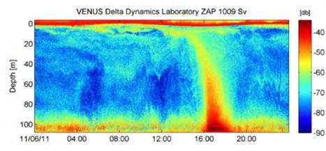
Ocean Networks Canada has been operating ASL's upward looking sonars since 2007 on the Venus network. One of ASL's instruments, a single frequency 200 kHz sensor, was deployed in 100 m of water at the mouth of the Fraser River, Vancouver at their Delta Dynamics Laboratory. It was deployed to view sediment distribution.
