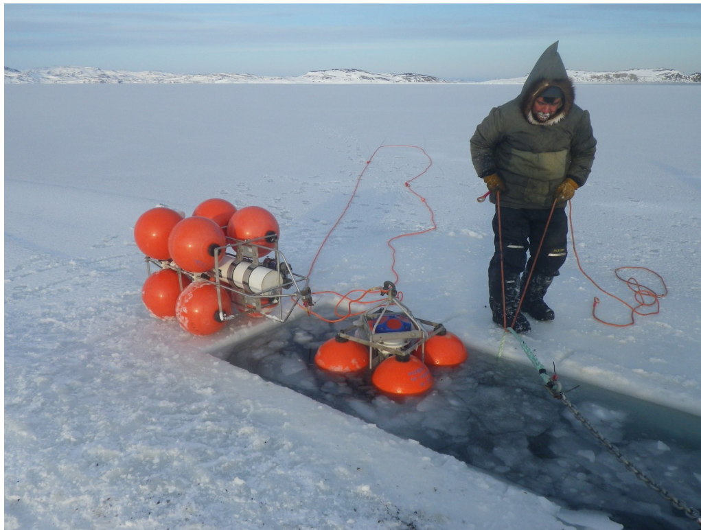
Joey Angnatok preparing ADCP and IPS mooring cages for deployment through the ice. (Photo credit: James Bartlett)
