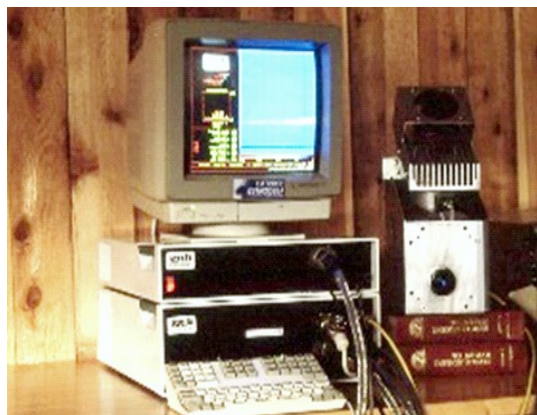
Figure 1. CASI (Compact Airborne Spectrographic Imager) —an instrument that changed the remote sensing paradigm.
