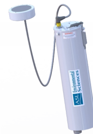
Figure 1. A high-frequency (455, 769, 1200 and 2000 kHz) Acoustic Zooplankton Fish Profiler (AZFP) autonomous echosounder to conduct observations of small zooplankton for ecosystem research.
