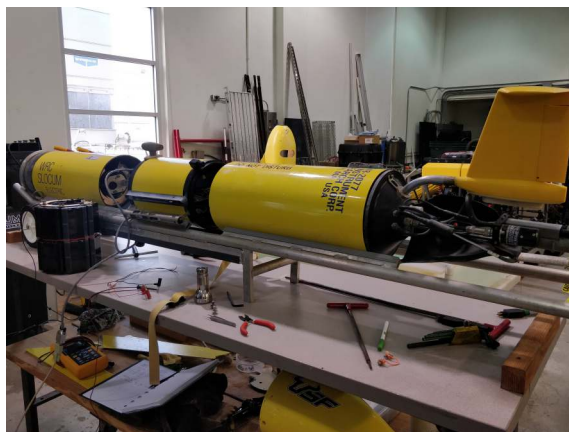
Slocum glider assembly showing the modular segments.
