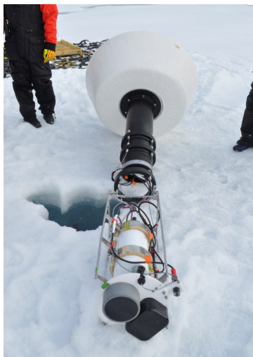
AZFP zooplankton sensor in its frame, attached to the buoy hull before deployment next to the prepared deployment hole in the sea ice.
