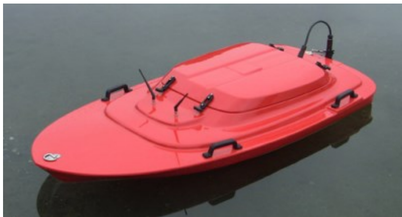
Teledyne RDI Q-boat fitted with a RiverPro ADCP.
