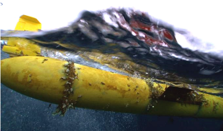
Photo of the Rutgers University's Scarlett Night Glider on its historic Atlantic crossing. Image shows barnacle-free areas where ClearSignal had been applied along with adjacent areas not treated. These non-treated areas at the seams of the glider's modular segments had, over time, bio-accumulations of barnacles.
