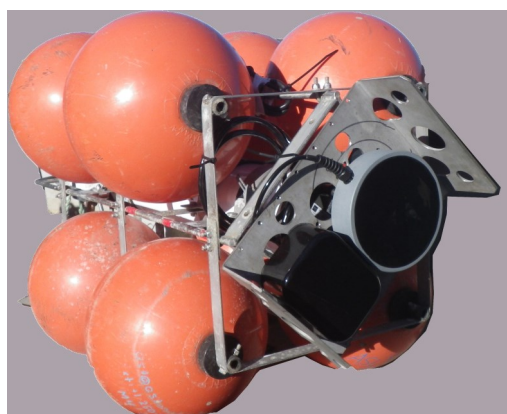
AZFP-ice deployment configuration. The black circular transducer is for the ice profiler and the black square transducer is for the multi-frequency calibrated echosounder. (Right)
