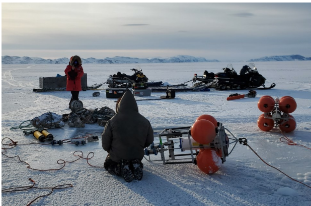
Through-the-ice deployment of the Log IPS on February 15, 2020. The Log IPS mooring cage is shown on the right along with an ADCP cage in the foreground to measure currents.
