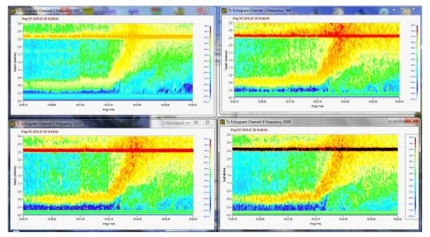
Figure 2. Acoustic backscatter data from all four frequencies (455, 769, 1250, 2000 kHz) during subsurface oil injections.
