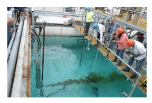
Figure 1. Subsurface oil release over AZFP.
