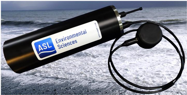
The unit uses nine common D-sized batteries with enough power for multi-week deployments. The instrument comes factory calibrated with a 200 kHz transducer with other transducers soon to be added. In the summer of 2024, the AZFP-nano was part of an International climate research expedition off the southeast coast of Greenland where it was used to collect 14 kilometers of water column data in a study focused on glacial-ocean interactions.
