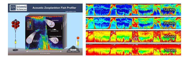
Acoustic Zooplankton Fish Profiler (AZFP) example mooring configurations and data time series.
