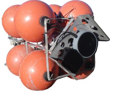
Diagram of AZFP6-ice deployment showing the ice and water column profiling capabilities. AZFP6-ice deployment configuration. The black circular transducer is for the ice profiler and the black square transducer is for the multi-frequency calibrated echosounder.
