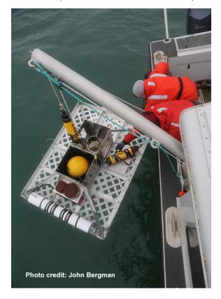
The AZFP was mounted on a low profile mooring frame and oriented to look upwards. It will record data continuously for a year and it is also equipped with a CTD and an adjacent current meter. These data will help detect the habitat parameters that may be associated with changes in fish and plankton distribution in the nearshore environment.
