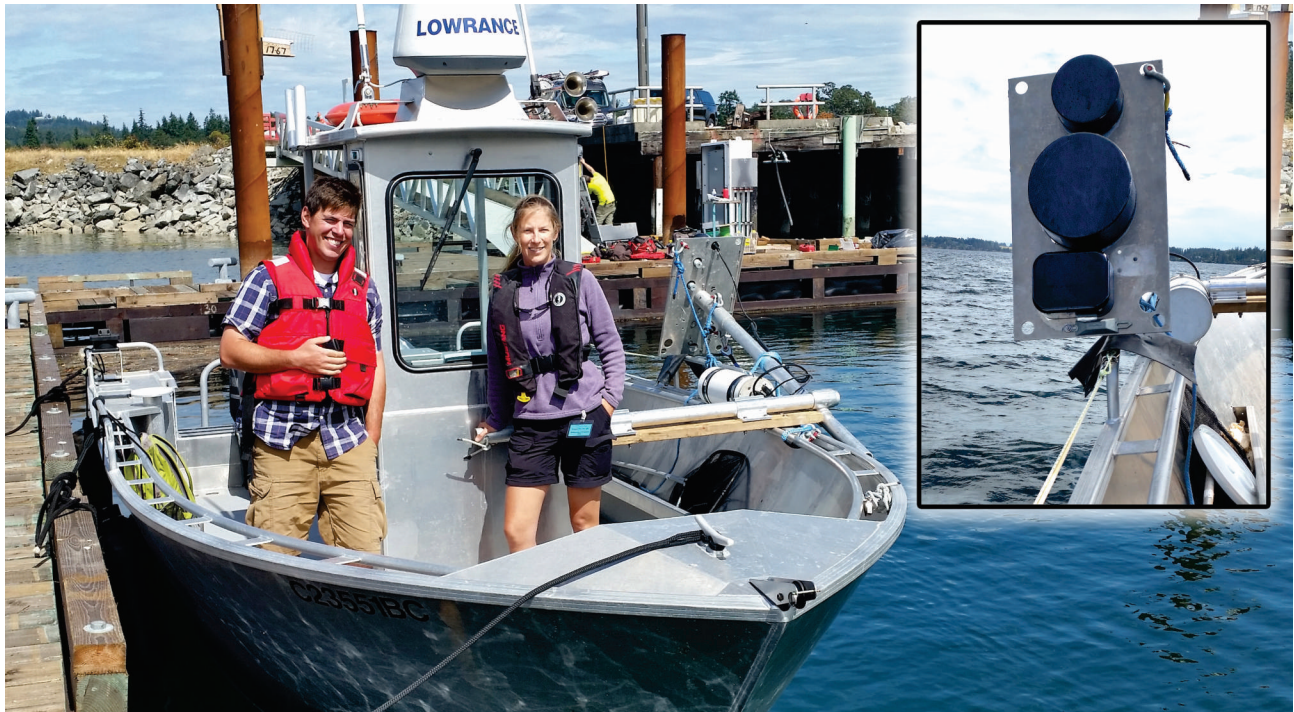
Ph.D. candidates Will Duguid and Rhonda Reidy with multi-frequency 38, 70, 125 and 200 kHz AZFP shown in inset
