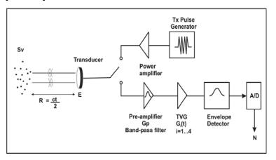
Figure 1. The generalized signal path for an Acoustic Water Column Profiler.
