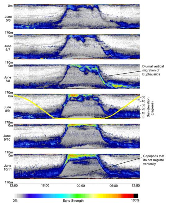
**Figure 3.** A week long series of echograms for June 2001, illustrating changes of vertical distribution of scatterers in Saanich Inlet, from minutes to days. Yellow line shows the approximate sun elevation on June 7. (Images have been grossly decimated for inclusion here. See reference 2, or contact the authors for higher resolution figures)
