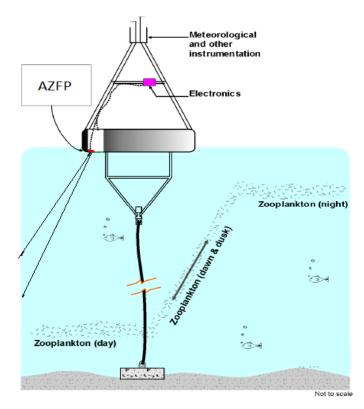
data from a moving platform such as this is not so "clean" as from a bottom mooring especially for smaller buoys and/or more dynamic seas.
