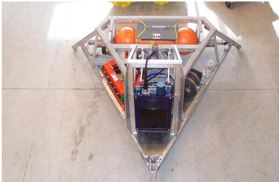
Figure A3-2. Bottom-mount package with Coda sonar installed (sonar head at front). SeaBattery is orange rectangular object on left (also provision for mounting 2 nd battery). DIU electronics is opposite battery on right. Acoustically released recovery float with associated line constitutes the orange dumbbell-shaped object near platform rear.
