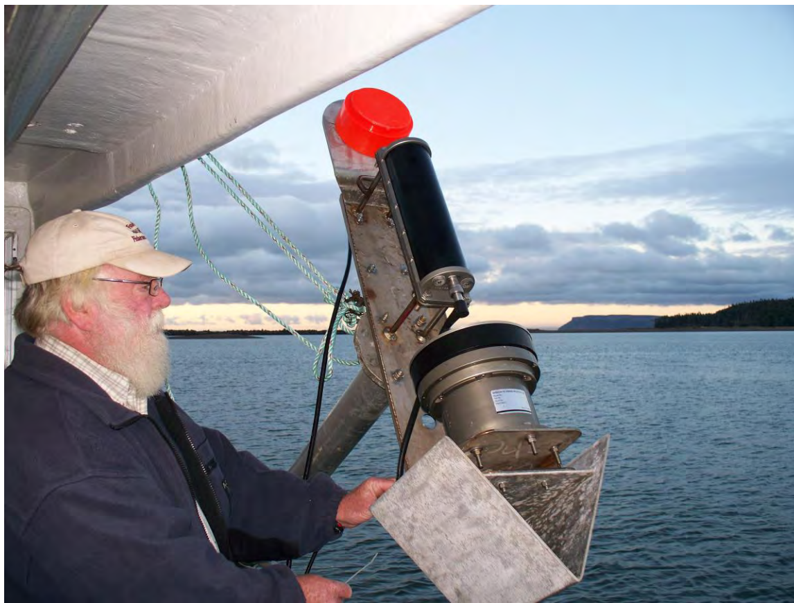
Figure 3. Boom-mounted acoustic transducer package attended by DFO Research Scientist G. Melvin. The orange unit at top is the 120 kHz Simrad EK60 split-beam transducer. Immediately below it lies the 200 kHz Kongsberg-Mesotech MS 2000 narrow beam, linear transmit transducer. Near bottom is the circular arc MS 2000 receive transducer.
