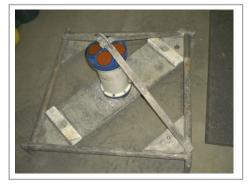
**Golder Associates** of Edmonton, Alberta leased a 300kHz RDI ADCP for measurements related to a mine and jetty development in Nunavut. ASL also provided a bottom frame that could be deployed from their small boat.
