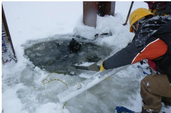
**Figure 3:** SWIPS with internal battery being deployed
