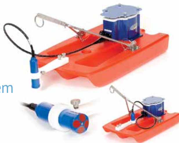
The StreamPro's transducer can be towed from the front or middle of the float, or can be removed and hand-held in the water for applications such as under-ice flow measurements.
