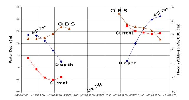
Fig. 3. *Norton* sensor data during the lower low tide of April 22, 2003. The gap is the in-air period when the water level was below the sensors.
