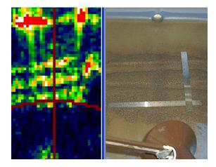
Fig. 2. Imagenex sonar image (left) of a set of three test sand ripples (about 1-2 cm height, and 10 cm length) in a tank.
