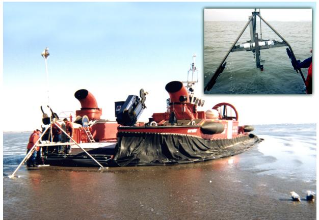
Fig. 1. *Norton* being deployed on Roberts Bank using the Canadian Coast Guard hovercraft *Siyay*. A relatively easy deployment, and we knew that it was deployed right-side-up. Insert shows the tripod being recovered. Two OBS sensors were attached to the legs, while the Imagenex scanning sonar (red head) and the Marsh McBirney flow sensor (black ball) were mounted in the centre of the tripod.
