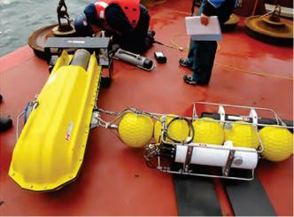
The Ice Profiling Sonar (left) and current meter node (right) being deployed in the Strait of Canso. (photo credit Jim Hamilton)
