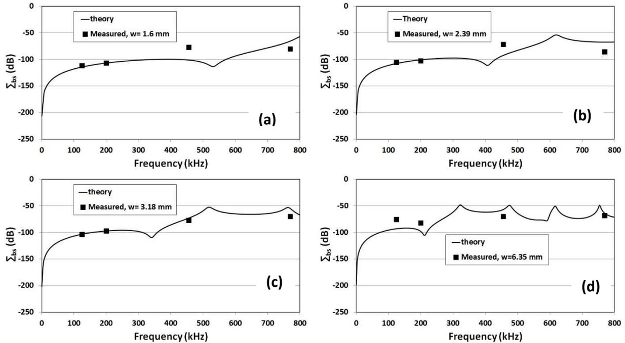
**Fig. 4.** Plots of theoretical and measured values of  $\Sigma_{bs} = S_v$  as a function of acoustic frequency for brine suspended Glitter particles with widths ( $w$ ): a) 1.6 mm; b) 2.59 mm; c) 3.18 mm; and 6.35 mm. “Theory” values were calculated using Eqs. 2-4 in conjunction with the corresponding “effective radii” of the particles.
