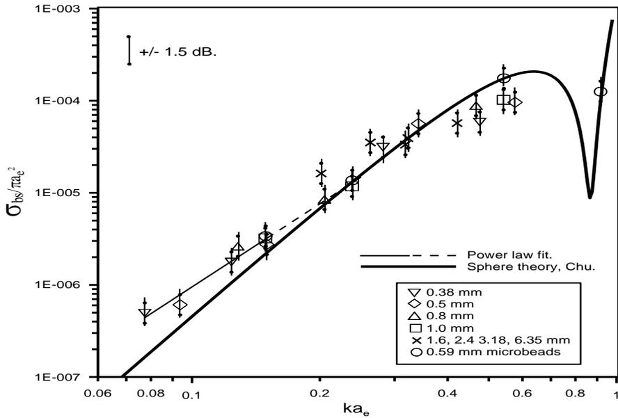
**Fig.5.** Deduced backscattering cross sections (normalized by dividing by  $\pi a_e^2$ ) plotted as a function of  $ka_e$  for the indicated disk diameters and the microbead spheres. The included curves represent an optimized power law fit and theoretical expectations based upon the Chu algorithm and the Faran Theory.
