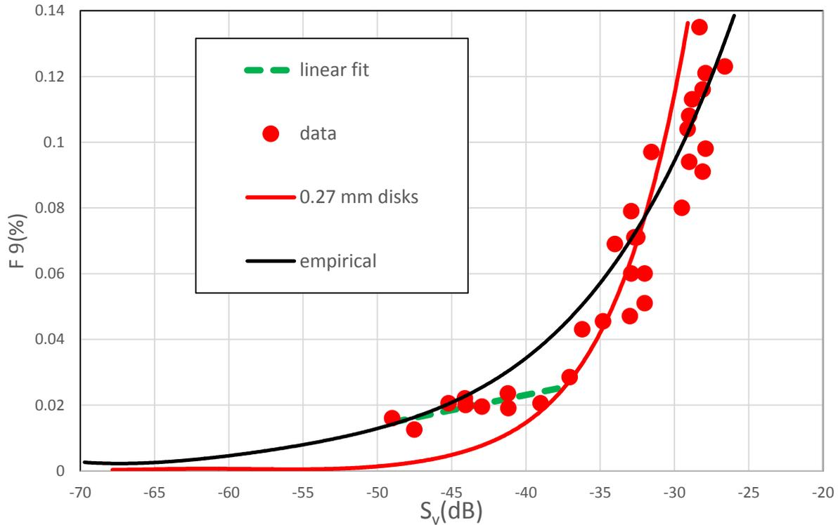
**Fig.1.** (Adapted from Ghobrial, 2012) Plots of UAWRE test tank frazil fractional volume ( $F$ ) vs. backscattering coefficient ( $S_v$ ) data and a resulting least square “empirical” regression fit to Eq. 6. Additional curves include a linear regression applied to data points for  $F < 0.03\%$  and a curve to represent optimal theoretical ( $F, S_v$ ) results calculated for using the Coussios (2002) theoretical cross section for a population of identical frazil disks of radius=0.27 mm.
