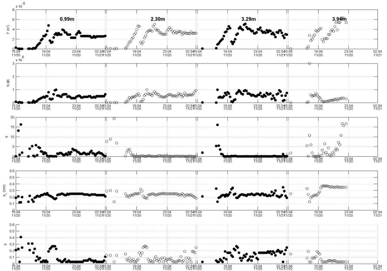
**Fig. 7.** Plots of frazil parameter,  $F$ ,  $N$ ,  $q$ ,  $a_m$  and  $b$  values corresponding 4 indicated measurement range as derived from RUNSWIPS extractions carried out on SWIPS channel 1, 3 and 4 data from the Nov. 20-21 frazil interval . Data was limited to ranges centred no further than 3.94 m from the transducer plane to avoid interference with near-surface ice.
