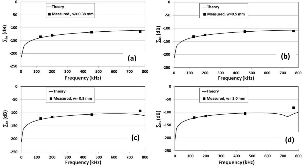
**Fig. 3.** Plots of theoretical and measured values of  $\Sigma_{bs}$  (equivalent to  $S_v$ ) as a function of acoustic frequency for brine suspended Glitter particles with widths ( $w$ ): (a) 0.38 mm; (b) 0.50mm; (c) 0.80 mm; and (d) 1.00mm. “Theory” values were calculated using the Faran (1951) formulation in conjunction with the corresponding “effective radii” of the particles and the optimal polystyrene sound speed parameters.
